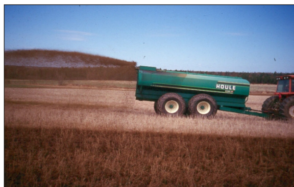
The largest losses of \text{NH}_3 occur with top discharge manure spreaders utilizing splash plates.
